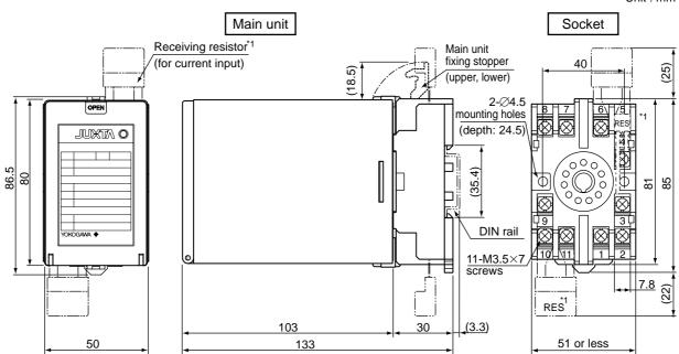
\*1: The receiving resistor is supplied for the input signal suffix code "A"
